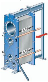
Step 2: After that bolts are tightened alternately and diagonally, as shown in the figure below. Check the dimension A during tightening at the positions of the bolts that are being used.
