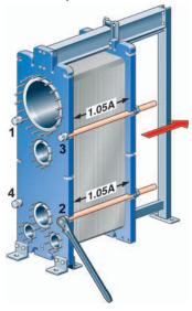
Step 2: Loosen the two diagonal pairs of bolts are loosened alternately, as shown in the figure below.
